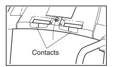
To measure your heart rate, stand on the foot rails and hold the metal contacts on the handrail—avoid moving your hands. When your pulse is detected, the heart symbol in the right side of the display will appear, one or two dashes will appear, and then your heart rate will be shown. For the most accurate heart rate reading, continue to hold the contacts for about 15 seconds.
